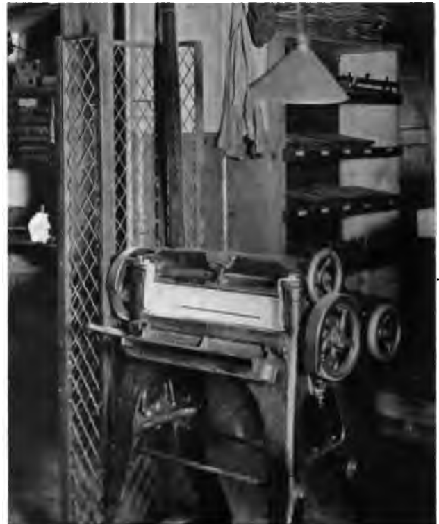
Fig. 4. Skiving Machine with Rolls and Belt thoroughly protected.*
